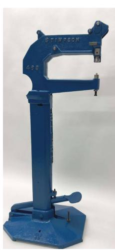
The 469 foot press is a manual feed machine used for limited production runs. With the proper tooling installed it can set eyelets, grommets, rivets, snaps, clamps, spots and many other small findings. The machine has a 10.25 inch throat depth which setting fasteners in larger objects. The 469 machine's double lever system and larger foot pedal make it easy on the operator to install fasteners with less fatigue with extended use. An air assisted version is also available.
