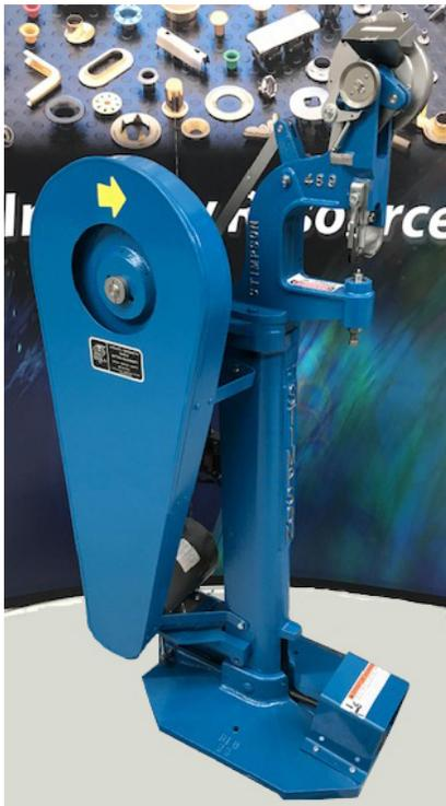
**Size Capacity:** 1/8 inch diameter eyelets to a 1/4 inch eyelet or grommet
