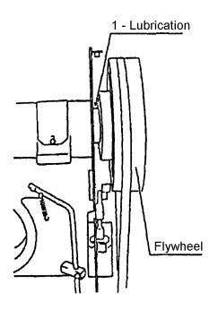
1) Remove the flywheel cover, and then apply 4 or 5 drops of oil to the shaft via the top of the clutch unit, while slowly rotating the shaft by hand.
