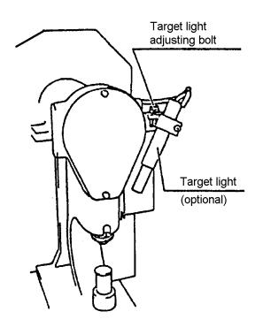
1) Loosen the target light adjusting bolt(s).
