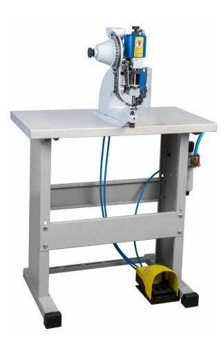
The J-230 is a pneumatic powered single feed rivet machine capable of punching and setting rivets into leather, cloth, plastics, nylon webbing and most other materials. The machine punches and sets in one stroke. The machine will either score set or roll set the rivet depending on the bottom die you use. Like all auto feed machines, the J-230 is set up to run one size rivet only but has the capability to run different length barrels of the same size rivet.
