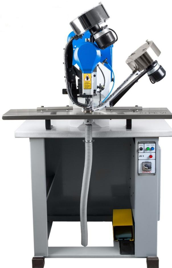
**Size Capacity:** #00 thru #4 grommets and washers
