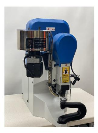
The J-380 is an electric powered single feed boot hook machine capable of punching and setting boot hooks into most leather. This machine was designed specifically for the shoe industry, but can be used for other applications as well. The J-380 comes complete mounted to a stand with a safety devise and laser pointer. The machine punches and sets in one stroke. Like all auto feed machines, the J-380 is set up to run one size boot hook only.
