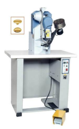
The J-569A & J569B are electric dual auto feed snap machines setup for industry snap fastener components. The J-569A feeds and sets the Cap and Socket parts of the snap and the J-569B sets the Stud and Post parts of the snaps. These machines are usually sold in pairs as two machines are needed to feed all four parts of the snap set. The machine punches a hole and sets the two part snap in all types of materials including leather, vinyl, plastics and textiles.
