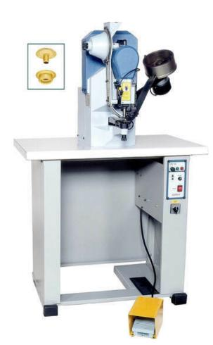
The J-569B & J569A are electric dual auto feed snap machines setup for industry snap fastener components. The J-569B feeds and sets the Stud and Post parts of the snap and the J-569A sets the Cap and Socket parts of the snaps. These machines are usually sold in pairs as two machines are needed to feed all four parts of the snap set. The machine punches a hole and sets the two part snap in all types of materials including leather, vinyl, plastics and textiles.
