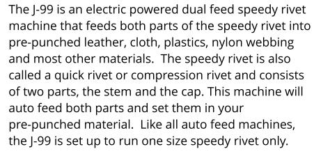
**Size Capacity:** The J-99 can be set up to run most popular size speedy rivets from 1/8 inch to 9/64 inch
